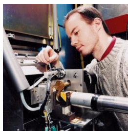
Figure 6. the shear cell on the LOQ Instrument at ISIS in the UK. The incident neutron beam enters from the right, the window to the detector is visible on the right.
